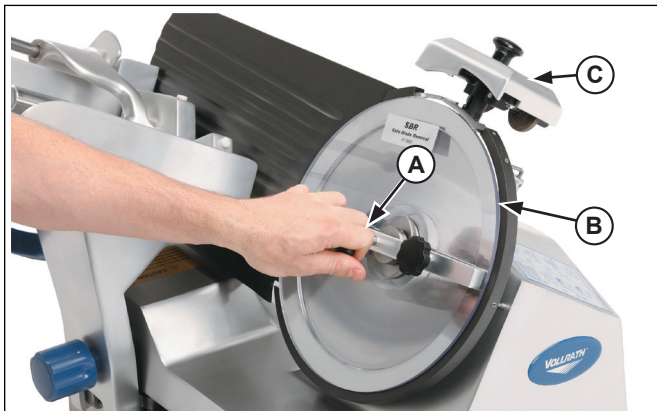
Figure 4. Safe Blade Removal Tool and Blade and Sharpening Assembly
