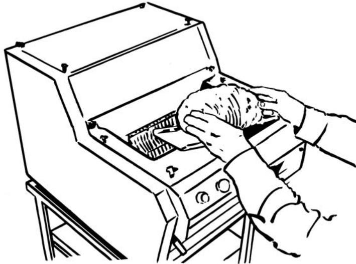
The bagging scoop's bread stop is adjustable to accommodate various size loaves. To adjust, apply pressure to the outside edges of the bread stop and slide along the scoop to the desired position.
