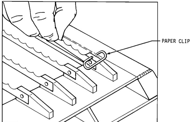
The blades can be removed from the lower blade frame while it is still in the machine. This is done by using a second special blade changing tool. Insert the tool into the blade frame, push the handle toward the feet of the blade frame as shown below. This will reduce the tension on the blade so that it can be carefully removed.
