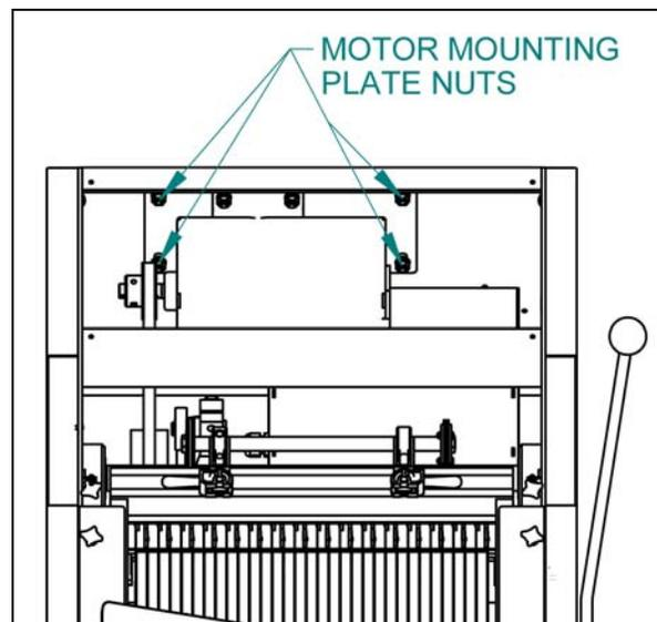
Manually lift the motor upward to tighten the belt using care to keep the centerline of the motor perpendicular to the centerline of the belt. The belt can be loosened by carefully moving the motor downward. The drive belt should be just tight enough, using moderate finger pressure, to allow a 3/8 inch deflection halfway between the motor drive pulley and the driven pulley. When desired belt tension is achieved, retighten the motor mounting nuts securely and replace the top cover.
