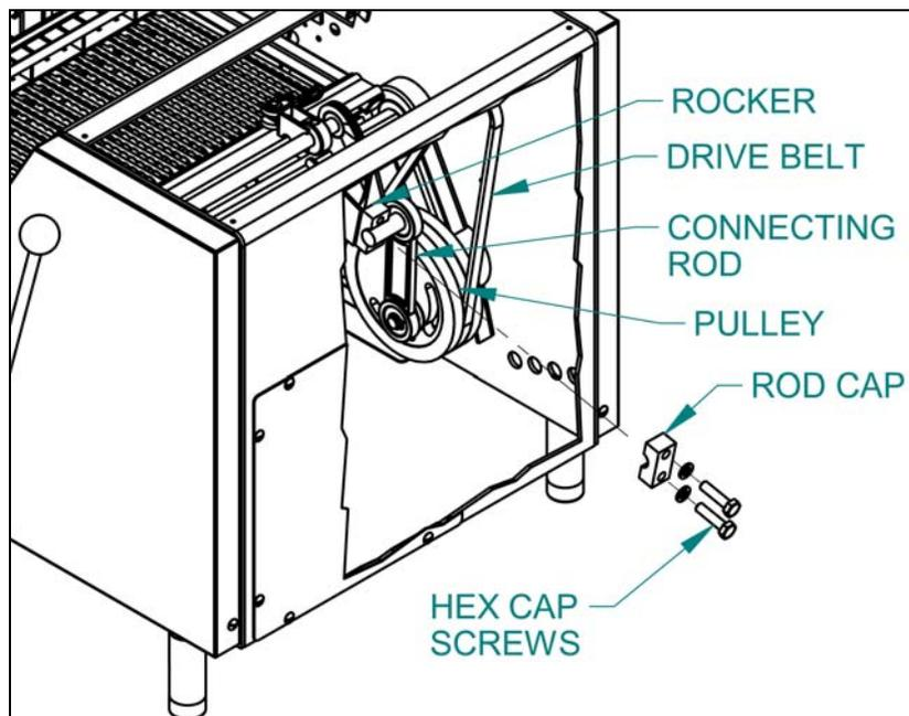
After replacing the belt reattach the connecting rod making sure to place the connecting rod as perpendicular as possible to the rocker's main shaft. Retighten the rod cap's bolts securely. Tighten the belt as described in the "Tightening the Belt" section of this manual and then replace the top cover.
