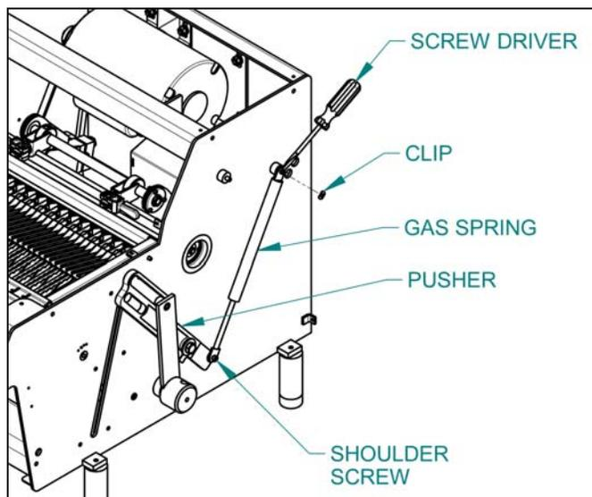
Install a gas spring by first attaching the lower end of the spring to the pusher arm with the shoulder screw.
