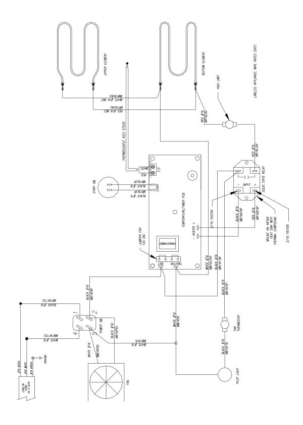
CABINET WIRING IS #16AWG MGT, CSA STYLE A-24, 26/30 STRAND TYPE A NICKLE
