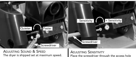
ADJUSTING SOUND & SPEED The dryer is shipped set at maximum speed. Turn counterclockwise to reduce sound and speed. 3/4 of a turn max. ADJUSTING SENSITIVITY Place the screwdriver through the access hole as shown to adjust sensitivity. Range is set at the factory for 4 - 6 inches.
