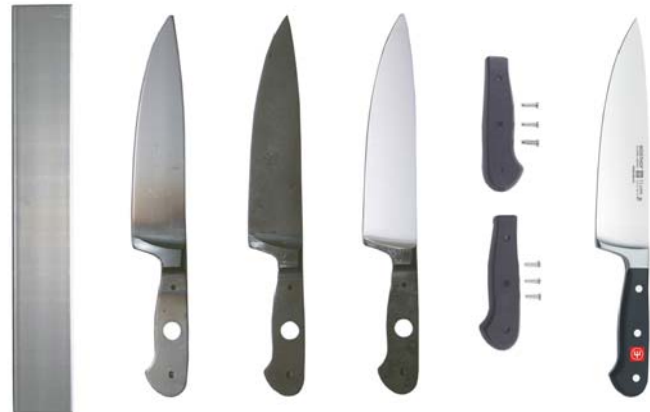
1 Sheet bar of high carbon no-stain steel 2 Precision forged piece 3 Tempered to 58° Rockwell 4 Polished 5 Scales of handles and rivets 6 The WÜSTHOF Cook's Knife
