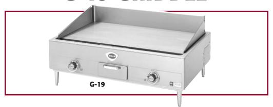
Wells Griddle G-19 is ideal for any kitchen based on its versatile, easy-to-use design. In addition to the standard grill surface there are two options to choose from, grooved or chrome-plated. The two positive-off thermostats allow individual zone control. The oversize grease drawer is easily removable for cleaning.
