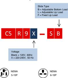
For Standard Voltage Cabinets (120V, 5.3A, 60Hz, 640W)
